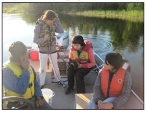
Students using a water thermometer to measure the temperature of the lake at different levels.
